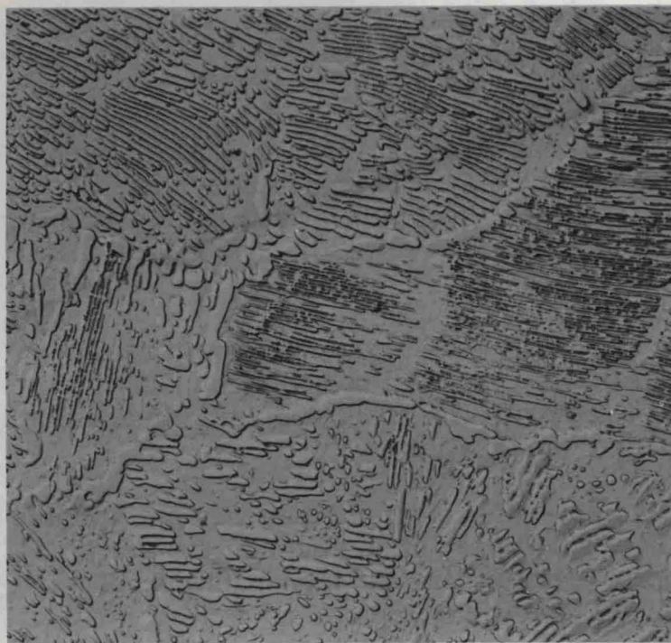
Fig. 28 0.92 per cent carbon high-purity steel held for 1 minute at 600°C at a pressure less than 500 atm, etched in picral. Electron micrograph, shadow-cast carbon replica. 7000X
