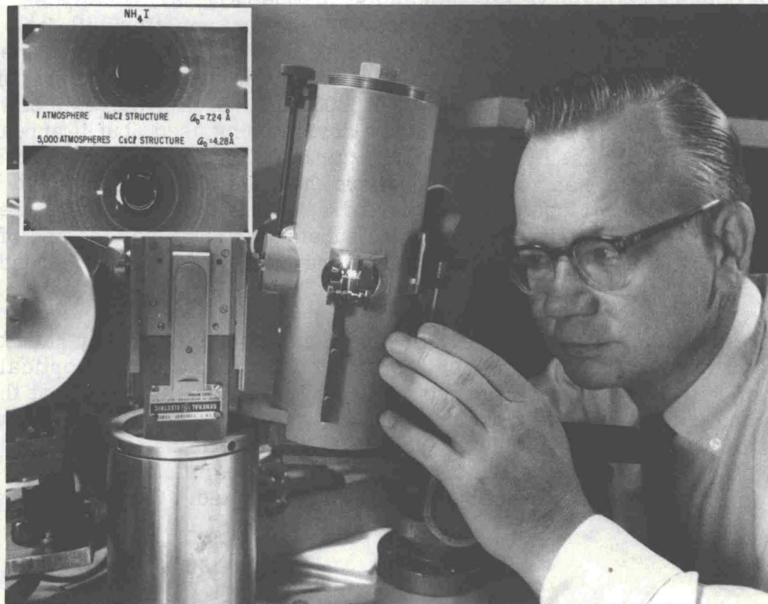
Fig. 20 High-pressure diffraction apparatus being adjusted for high-pressure experiment.
