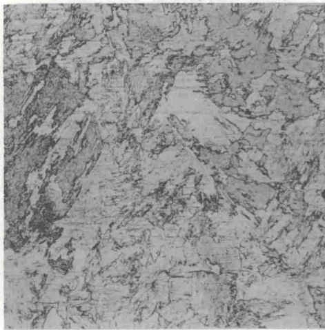
Fig. 2 Iron-(10 wt per cent chromium). Quenched after holding for 30 minutes at 1100°C, atmospheric pressure. 100X
