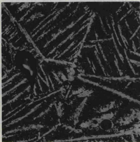
Fig. 9 Titanium-(10 wt per cent magnesium). Prepared by melting powdered components at 1900°C, 100,000 atm and cooled under pressure. (Globules of magnesium in an acicular titanium matrix.) 500X
