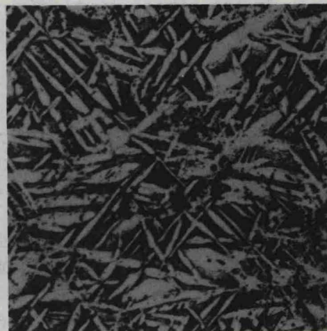
Fig. 10 Titanium-(2 wt per cent magnesium). Prepared by melting bulk components at 1900°C, 100,000 atm and cooling under pressure. 500X
